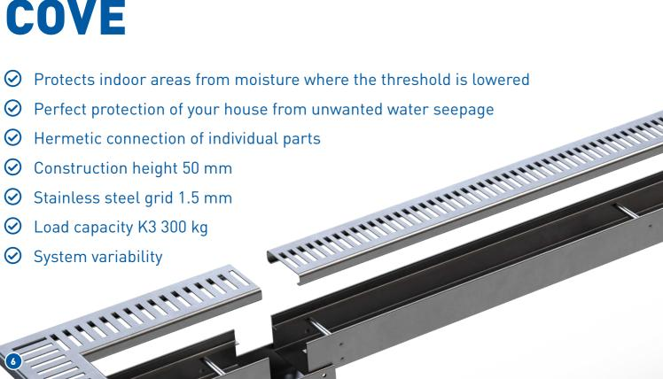
It safely ensures fast removal of extreme rainfall in sensitive areas such as door structures, terraces and balconies.
