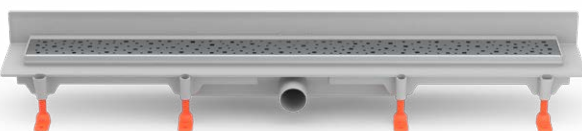
Linear floor drain D40 against the wall side outlet, with plastic frame
